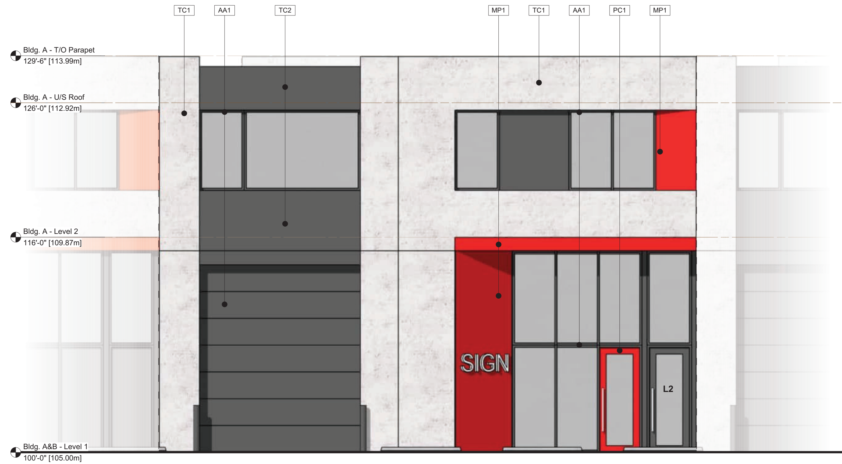
Building A Typical Unit Elevation
